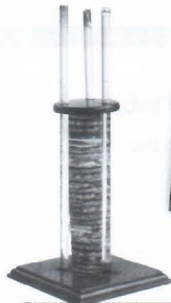
1 The first electric battery
